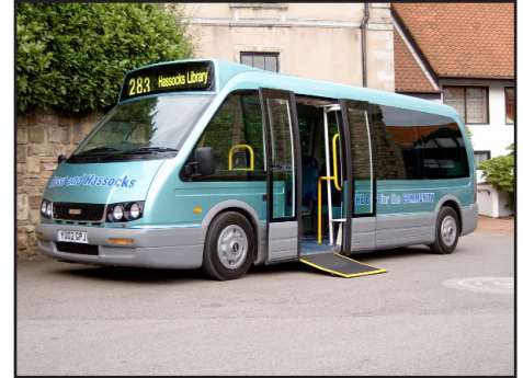
The Alero's ultra-low, flat interior floor combined with kneeling and lifting capabilities at both front and rear make it ideal for riders requiring easy access. When lowered, the entrance step is a mere 190mm (7.410") off the ground.
