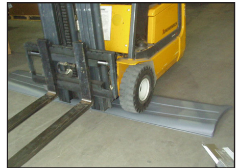
"To demonstrate the durability of KYDEX® sheet components to customers, we ran over one of the side panels with a 4-ton forklift, and the panel resumed its original shape," says Glenn Saint, technical director at Optare. When put to the same test, an ABS part shattered, adds Thompson Plastics' Paul Rhodes.
