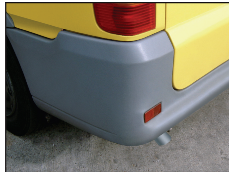
The use of colour-impregnated, impact-resistant thermoplastic on the Alero's bumpers and skirts minimizes visibility of scrapes and scratches common in low-profile buses.
