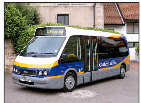
Colour-impregnated thermoplastic sheet used on the bumpers and skirts enhances the car-like style of Optare's Alero bus.
