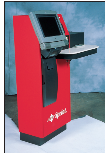
Exterior panels of Sprint bill payment kiosk membrane pressed with KYDEX® impact resistant sheet withstand more punishment than previous sheet metal units and, if damage does occur, allow fast replacement in the field at low cost.
