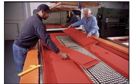
Operators remove panel from membrane pressing machine.
