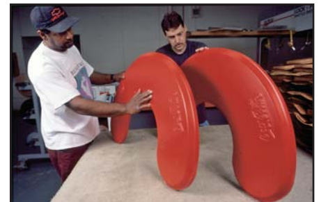
KYDEX sheet conforms to all top and side surfaces of three-dimensional substrates which, in this case, consist of doubled MDF board with injection molded Coca-Cola® logos affixed prior to membrane pressing, allowing seamless reproduction of corporate identity that resists damage.
