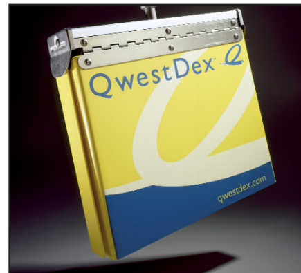
Telephone directory binders of KYDEX® sheet, an aluminum spine, and spring-loaded stainless steel hinges close in clamshell-fashion to minimize effects of weather, vandalism and wear.
