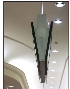
The clamshell design presents two halves, one slightly smaller than the other. The sides slip into one another and are secured by a thin extrusion. Depending on the location within the store, signs can be single- or double-faced.
