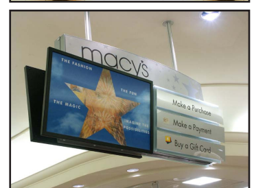
The centerpiece of the customer service sign is its 0.61m x 1.22m (2' x 3') lenticular graphics display, which employs a specially prepared (interlaced) image and a lenticular lens to produce a sequence of images. For instance, (above) a marching band plays within the star, while (below) fireworks explode. The display is pop-riveted to the clamshell for structural support.
