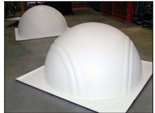
Thermoformed baseball halves await secondary operations at Piedmont Plastics, Burlington, NC
