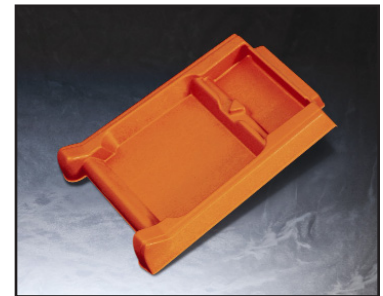
Thermoformed component incorporates indentations, stiffeners, and other details that conform to clearance and attachment requirements of finished part. Designers used wood and body filler materials to build the design prior to casting a mold for larger-volume production.
