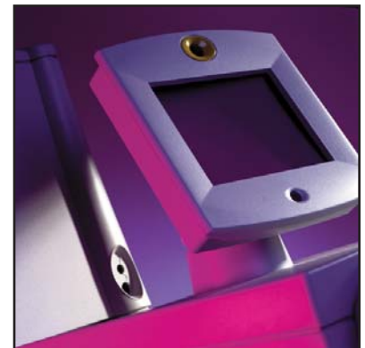
The housing is comprised of 17 components, all pressure-formed of KYDEX ® Vinyloy™ 103 thermoplastic alloy. For a quality finish, high strength and accurate fit of the finished assembly, parts must provide exceptional surface detail and uniform wall thickness.
